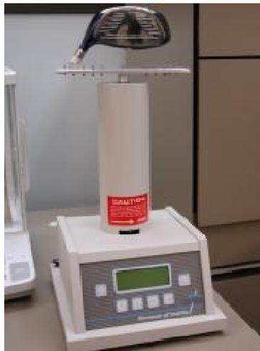
Diagram 3: Moment of Inertia Test Machine
